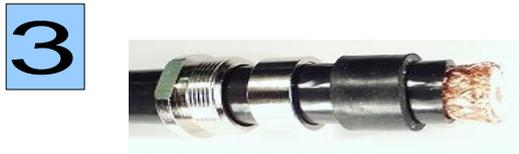
Remove 6 mm of the outer sheath with a knife.
