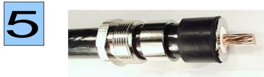
Remove the copper foil and the dielectric with a knife.
