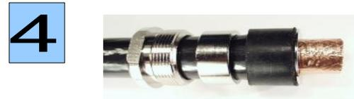
Bend copper braid upwards right-angled. Insert contact sleeve between copper foil and braid until stop. Cut off protruding braid. Move the rubber seal to the front, up to the contact sleeve.
