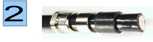
Move the nut, clamping ring and rubber washer over the cable tail. Hint: With a bit of Vaseline the rubber washer can be moved easily over the cable sheath.
