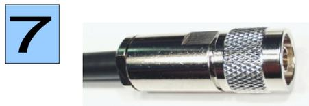
The prepared cable tail has to be inserted into the housing until stop. Tighten the clamping nut finger tight with two open-ended spanners 17/18 mm. A small split should remain visible between clamping nut and connector housing.
