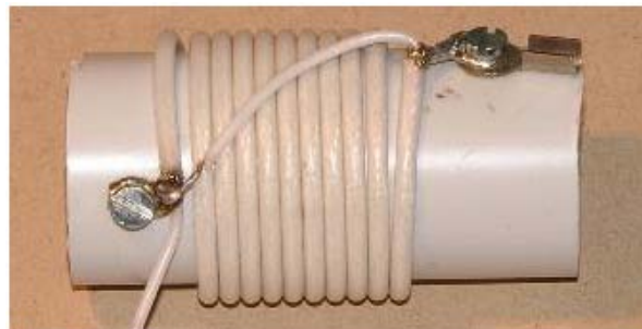
The picture shows a 30-m-Trap with PTFE-coax
