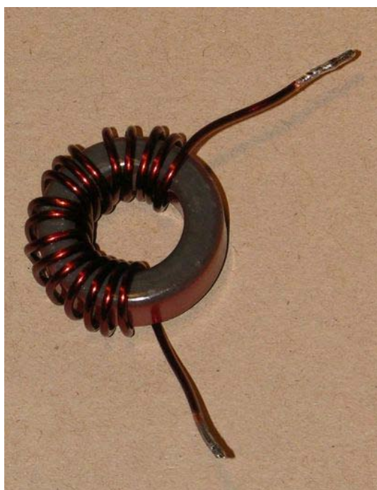
16 1/2 turns close spaced give an inductivity of 2,8 \mu\text{H}
