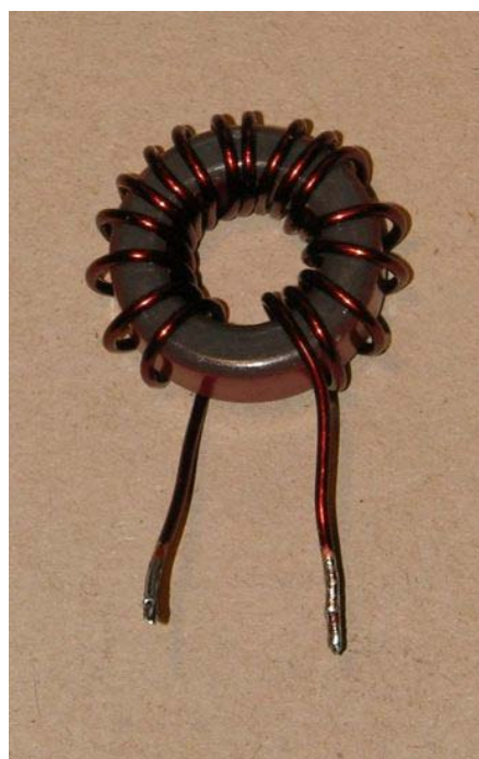
16 1/2 turns wide spaced give an inductivity of 2,5 \mu\text{H}
