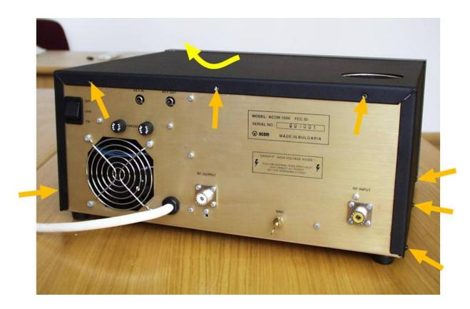
Lift the rear edge of the cover slightly (to 2-3cm) and then pull the cover backwards, in order to release it from front-panel's chutes. Remove the top cover.
