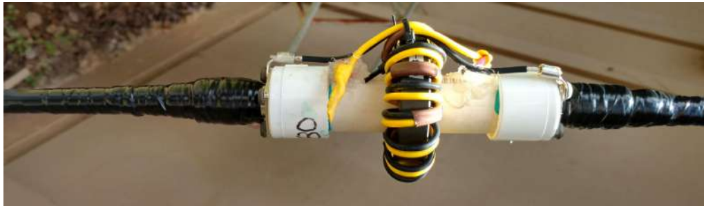
Fig 11 – W6GJB's Dipole Center Insulator With Two RG400 Chokes
