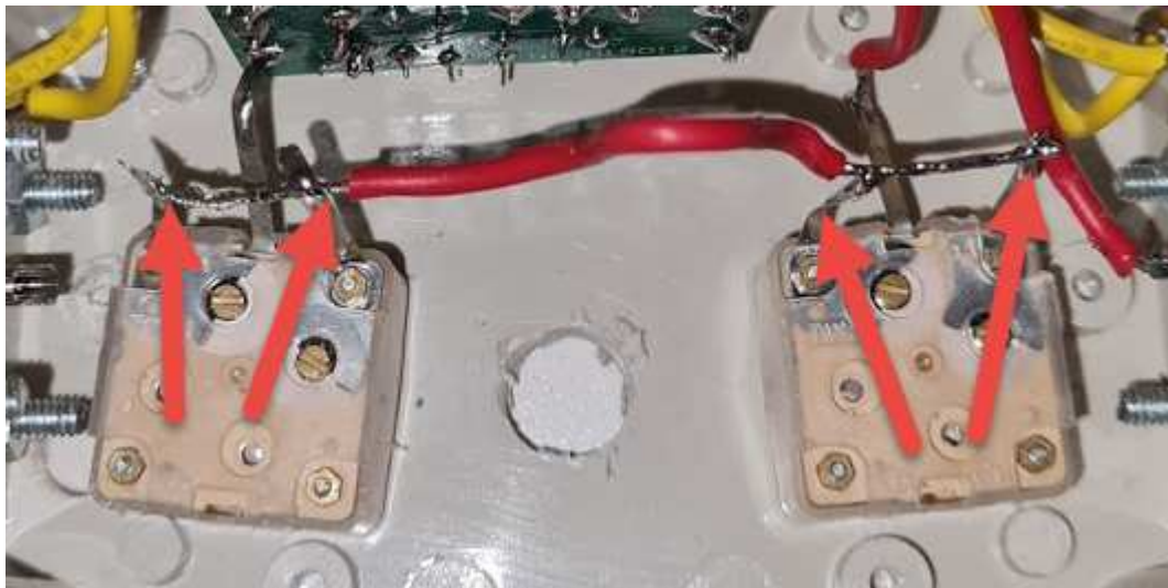
Figure 15 – Close up of the variable capacitor connections
