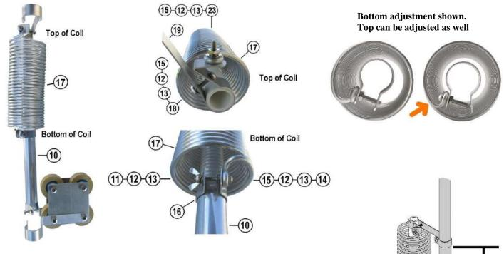
5. Install the TBR-160X assembly on the antenna, simply slide the free ends of clamps around the lower antenna element tube. At top of Coil snug the clamp in place - This will be adjusted during tuning.
