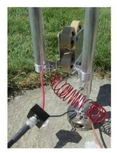
6. Connect the Q-Coil and the red lead of Feedpoint Connector to the bottom bracket for the 160 meter coil using the hardware as shown.
