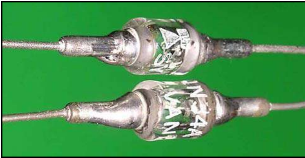
Diode Size (1/8" Diameter X 1/4" L) No Date Code
