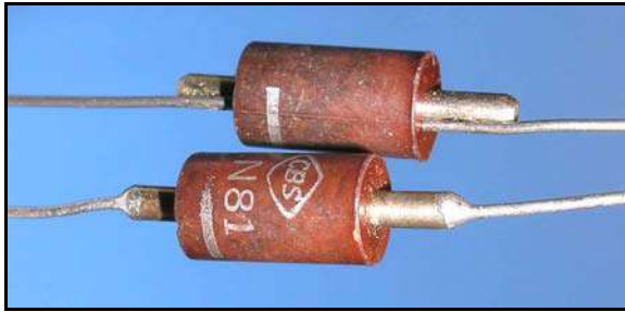
Diode Size (1/4" Diameter X 3/8" L) Date Code on Similar Units (1959)
