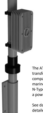
The AT-T is a broadband transformer with gain comparable to a commercial marine tuner. It has a 50 ohm N-Type female connector and a power rating of 150W.
